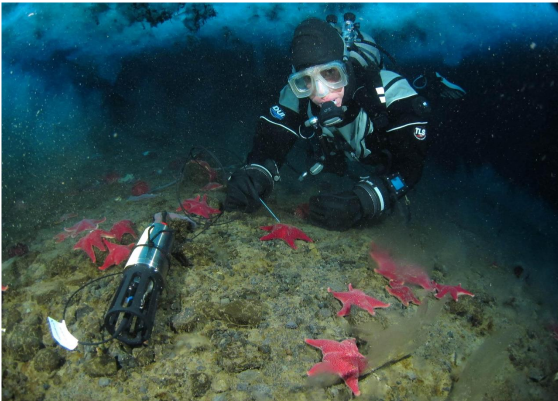
FIG. 1. Diver using AquaPHox-LX system with robust oxygen to measure oxygen at the surface of a healthy individual of the Antarctic starfish Odontaster validus . Photo by R. Robbins.
