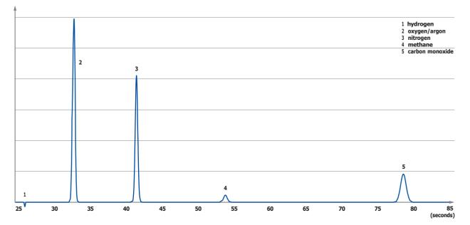
Example chromatograms: C<sub>1</sub>-C<sub>2</sub> NGA on P column (top left), C<sub>3</sub>-C<sub>5</sub>), H<sub>2</sub>S on U column (top right), BTEX on Wax column (mid) and H<sub>2</sub>, O<sub>2</sub>, N<sub>2</sub>, C<sub>1</sub> and CO on M column (bottom)
